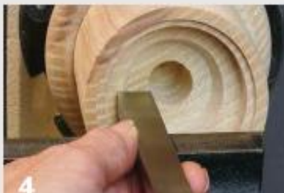
4 Hollow the inside of the box. (You are turning endgrain to make this box, so employ endgrain-turning techniques.)
