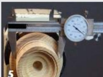
5 Transfer the measurement from the inside diameter of the bracelet to the outside diameter of the box so that the bracelet will slide easily over the outside of the box.
