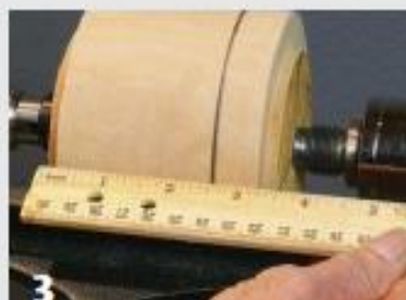
3 Turn a cylinder for the box and lid. Establish a tenon on each end. Mark measurements for top and bottom of the box.
